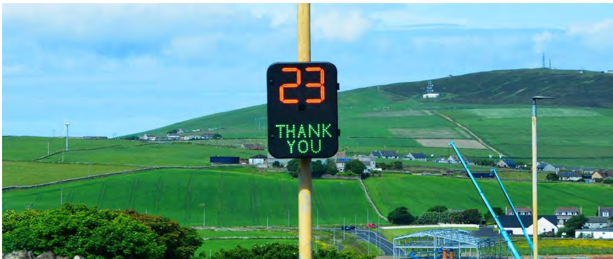
Figure 13 – Example of more expensive SID displaying vehicle speed
