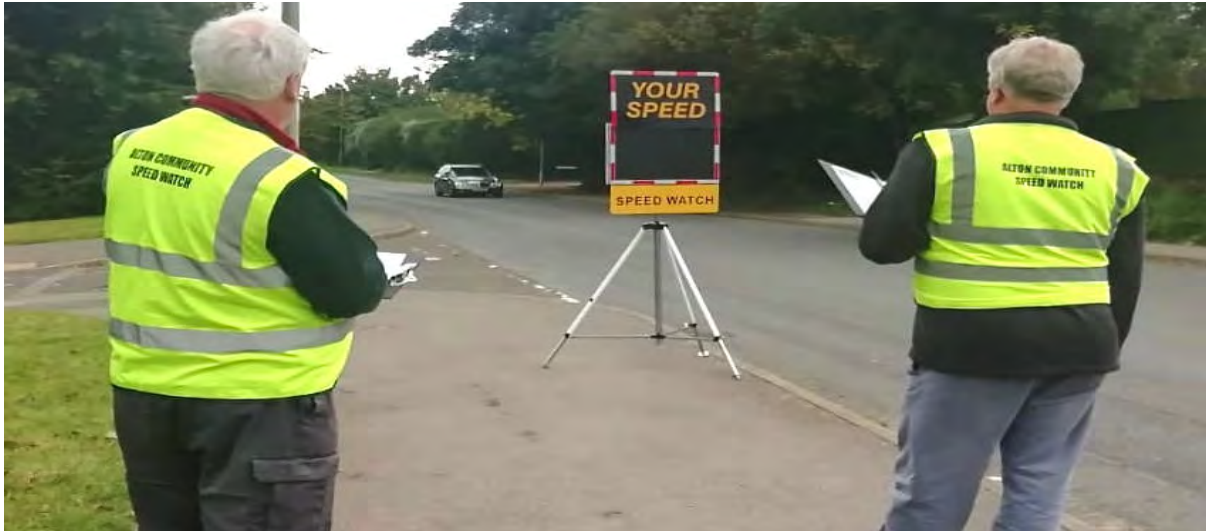
Figure 14 – Example of mobile VAS displaying vehicle speed
