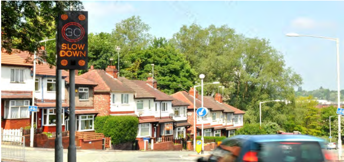
Figure 12 – Example of basic VAS displaying speed limit
